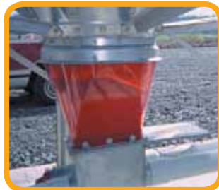
Polycarbonate boot transitions offer easy feed visibility.
