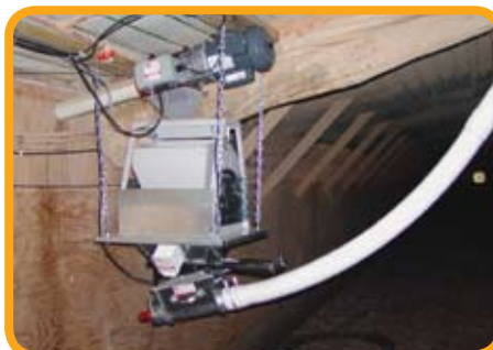
Chore-Time's Feed Scale aids in scheduling feed deliveries and provides real-time data regarding feed inventory.
